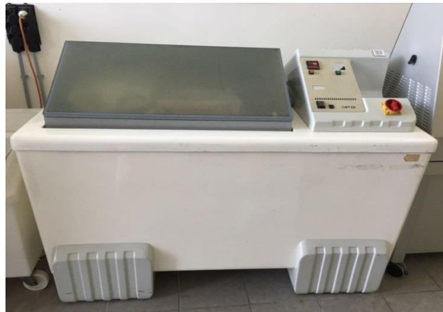
Figure 3.2. Humidity test cabinet at Şişecam (Ascott-H450T CTG 060)
