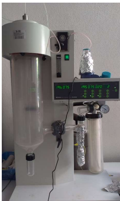
Figure 4. 3. Spray drying apparatus used in this study
