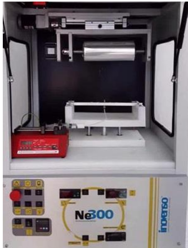
Figure 2.1 Electrospinning device (Inovenso Ne300)
