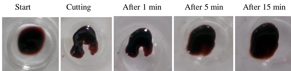
Figure 3.10. Gel form of (DOPA) 2 -PEG-(Trp) 2 (34 mM) with Fe 3+ (22.7 mM) at pH 9 in NaOH solution (0.5 M).
