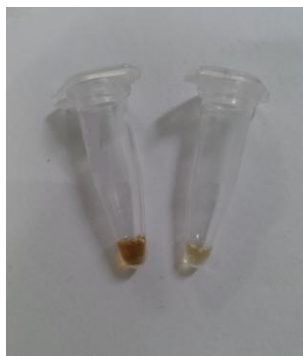
Figure 3.15. Gel form of PEG-(DOPA) 4 (8 mM) with IO 3 - (32 mM) in MES buffer (0.2 M, pH=3.0) (left), PEG-(DOPA) 4 (8 mM) with [IO 3 ] - (16 mM) in MES buffer (0.2 M, pH=3.0) (right).
