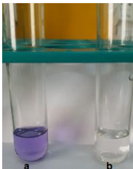
Figure 2.3. a) Positive primary amine test result of PEG-(NH 2 ) 4 , b) Negative primary amine test result of PEG-(N-Boc-L-DOPA) 4
