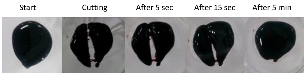
Figure 3.8. Gel form of PEG-(DOPA) 4 (17 mM) with Fe 3+ (22.7 mM) at pH 9 in NaOH solution (0.5 M).
