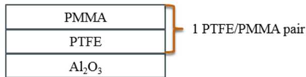
Figure 3.2. Film stack model of 1 pair PTFE/PMMA
