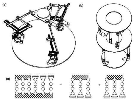
Fig. 2. (a) 6-dof spatial parallel manipulator with a triangular platform. (b)  $2 \times 3$ -dof modular spatial parallel manipulator. (c) Formation of a structural group using two simple structural groups.
