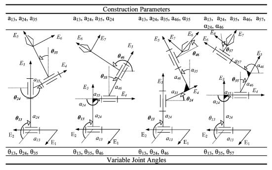
Fig. 3. Geometrical structural synthesis of an R-R-R kinematic chain.
