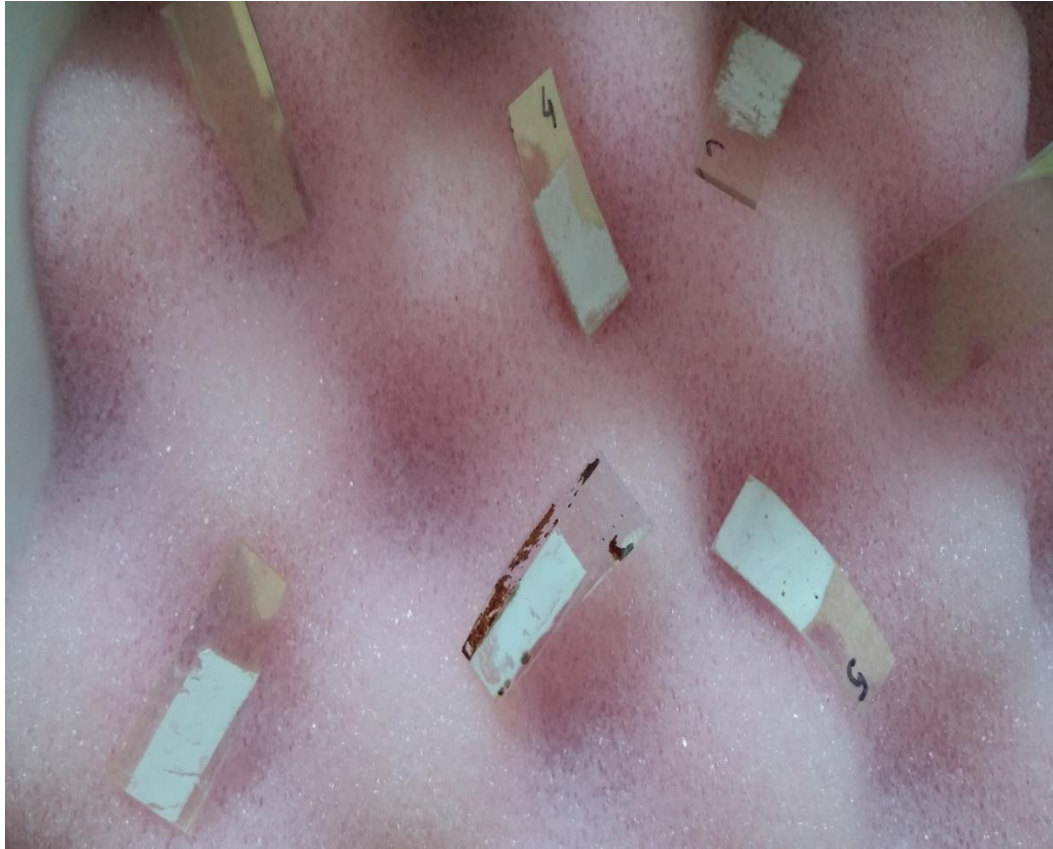
Figure 3.2. \text{TiO}_2 film coated ITO glasses prepared by doctor-blade technique.
