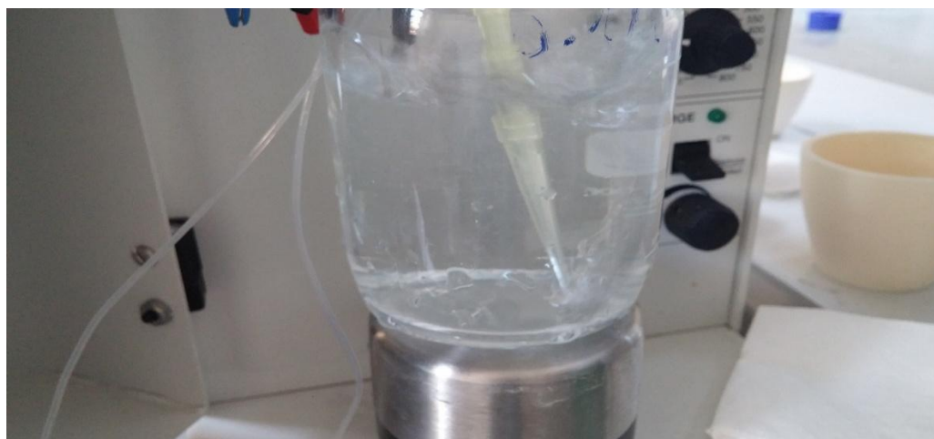
Figure 3.9. N 2 purging of 0.1 M KCl solution.
