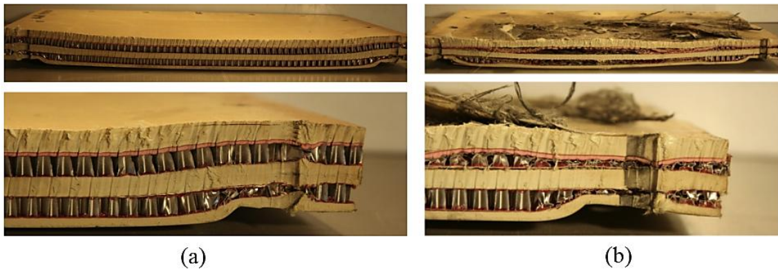
Figure 2.58. Deformation of double honeycomb core sandwich structures: (a) non-explosive blast test and (b) explosive blast test [101].
