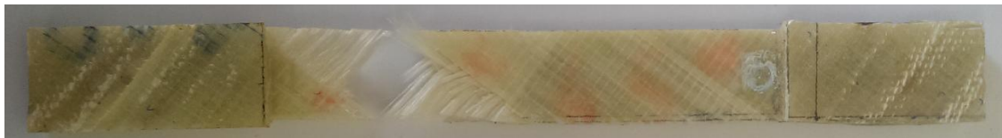
Figure 6.21. Failed composite sample after quasi-static shear testing.
