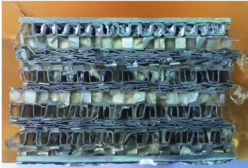
Figure 7.4. The quasi-static confined test sample compressed until about 0.4 strain.
