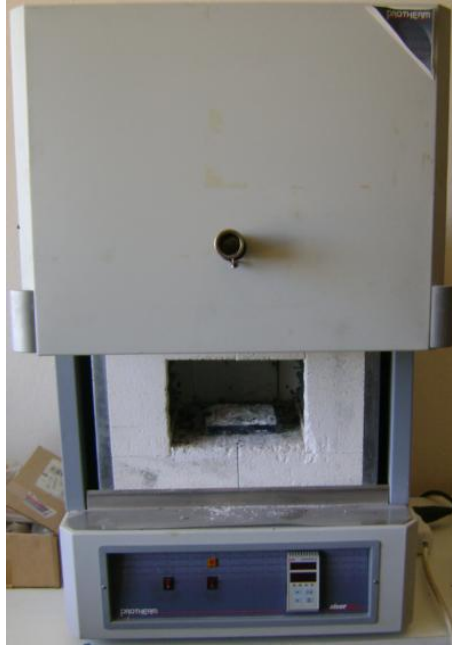
Figure 3.22. Furnace for heat treatment of 1050 H14 test samples.
