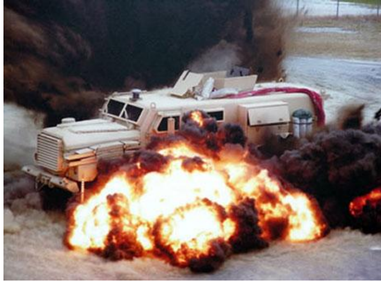
Figure 1.1. Full scale blast test of a military vehicle [1].
