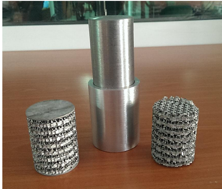
Figure 3.23. Constraint compression test apparatus and compression samples.
