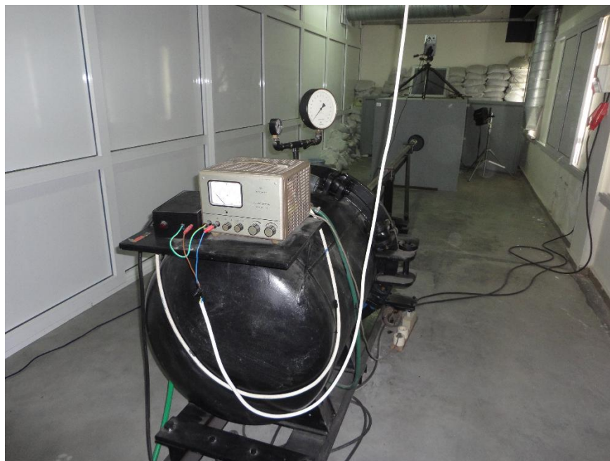
Figure 3.25. Projectile impact test set-up and high speed camera.
