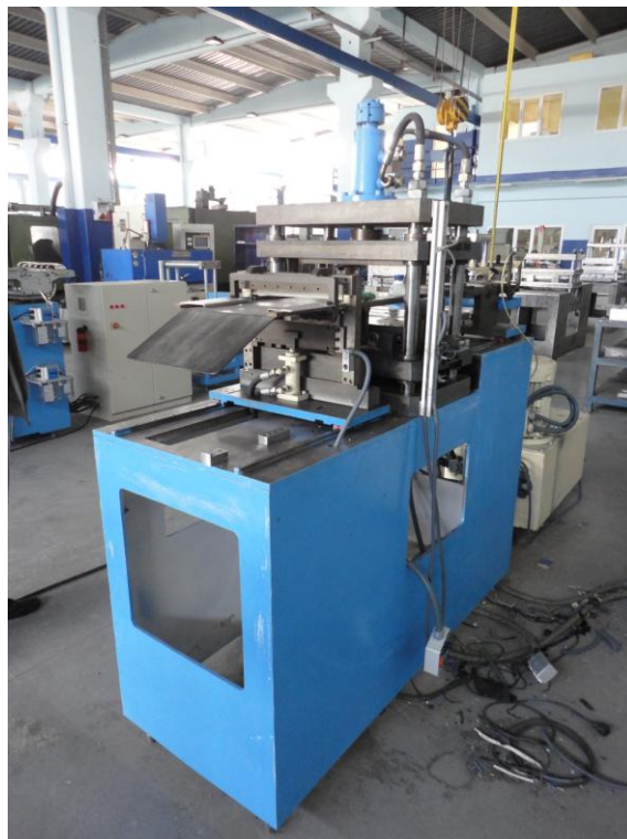
Figure 3.17. Hydraulic press used to form corrugated layers.
