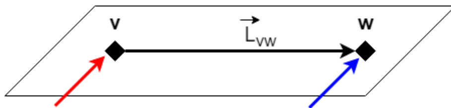
Figure 2.8 A rigid body defined by nodes v and w . The displacements of these nodes are given with dP_v , \delta_v , dP_w and \delta_w .
