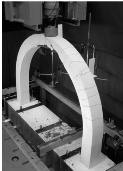
Figure 1.5. Pictorial view of the experimental setup (Source: Bhatti and Kishi 2011)
