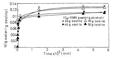
FIG. 4 Zeolite amount and the uptake curves.
