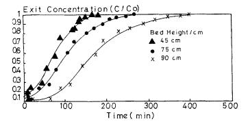
FIG. 8 Effect of packing height on the breakthrough curves.
