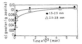
FIG. 5 Particle size and the uptake curves.
