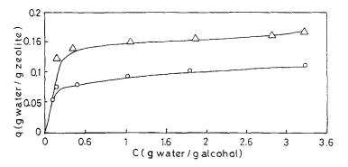
FIG. 2 Comparison of the adsorption isotherms of local clinoptilolite ( $\bigcirc$ ) and synthetic zeolite 4A ( $\triangle$ ).
