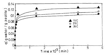
FIG. 6 Effect of temperature on the uptake curves.
