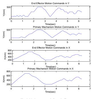
Fig. 5. Motion commands for end-effector and Primary mechanism
