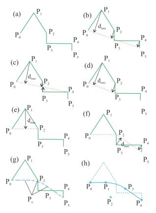
Fig.3. Corner reduction steps for a set of points.
