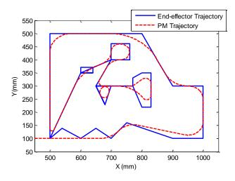
Fig. 4. Continuous motion commands generation for primary mechanism.
