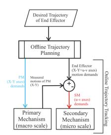
Fig. 1. Information flow of motion commands for redundant manipulator.
