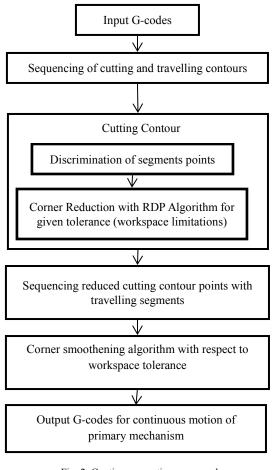
Fig. 2. Continuous motion commands generation for primary mechanism.
