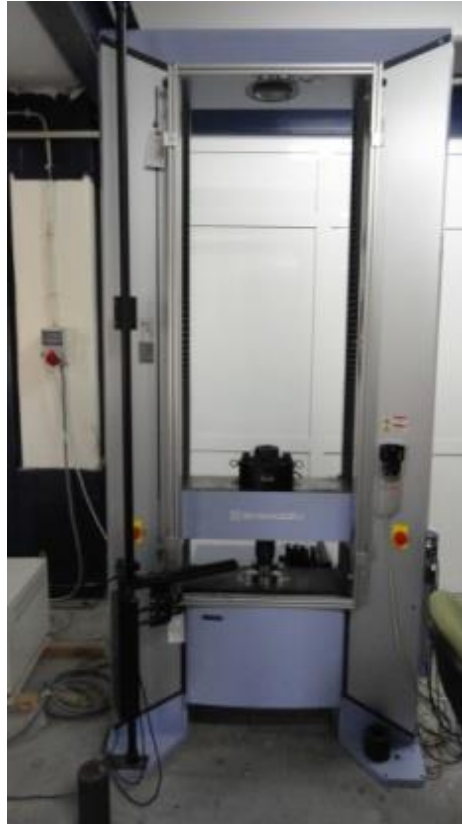
Figure 3.8. Shimadzu AG-X 300 kN universal testing machine.
