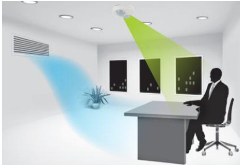
Figure 2.7. The integration of motion sensors and HVAC system. (Source: www.makelsmarthome.com.tr )
