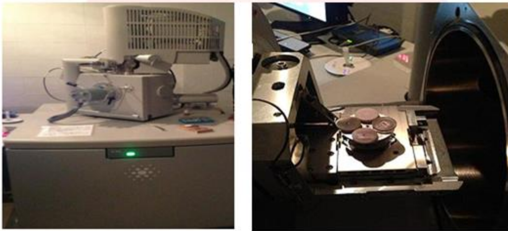
Figure 5.28. Image of a) scanning electron microscope (SEM) equipment b) polyester samples into the sem equipment
