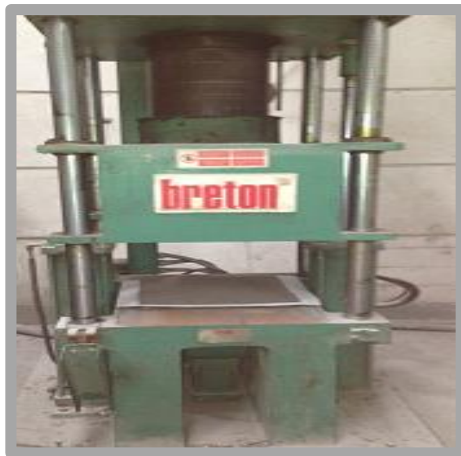
Figure 4.7. Vibropress machine used for polyester composite stone
