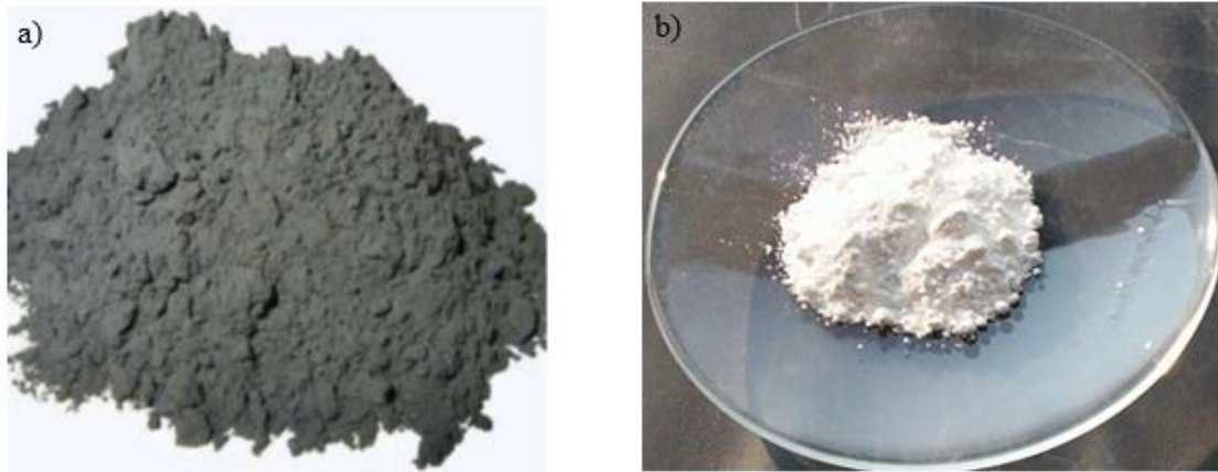
Figure 4.1. Antibacterial agents used with the study a) Silver powder b) Zinc oxide powder
