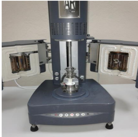
Figure 4.10. TA Instruments AR2000ex oscillatory rheometer used within the experiments
