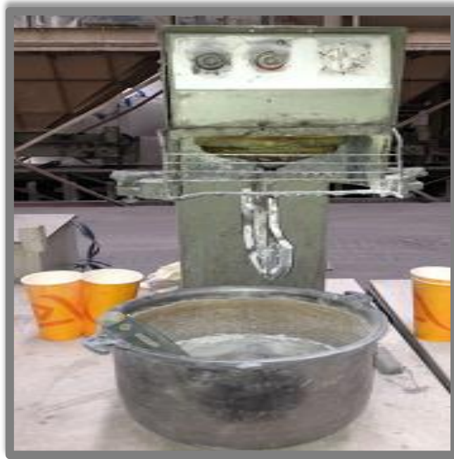
Figure 4.6. Homogenization of quartz nanoparticles and unsaturated polyester resin by homogenizer mixer
