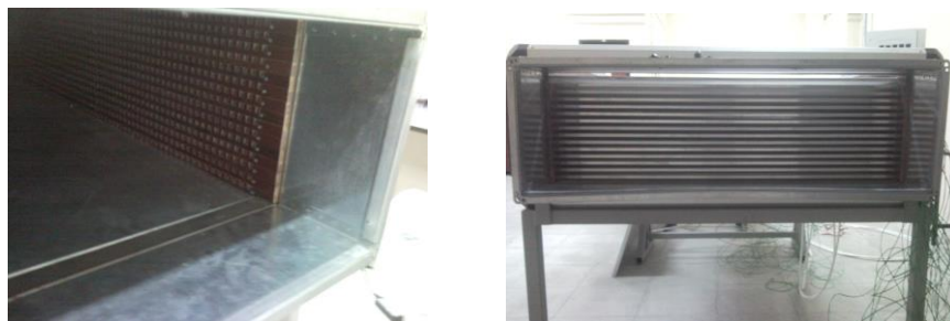
Figure 6.8. Outlet of the packed bed, a) wooden plates used for the placement of rods b) the located rods in the channel
