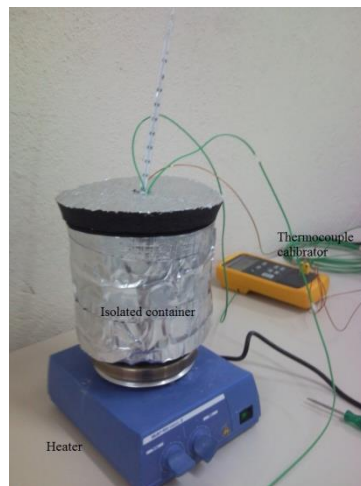
Figure A.1. Temperature calibration setup
