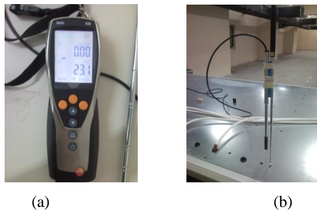
Figure 6.13. Velocity measurement device (Testo 435-2) (a) main device, (b) hot wire probe and a magnetic mechanism for the velocity measurement
