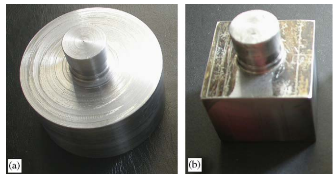
Fig. 6. Compression test apparatus for (a) hexagonal-packed and (b) square-packed multi-tube designs.
