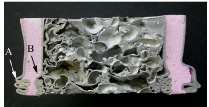
Fig. 11. Side view of crushed BPA specimen.
