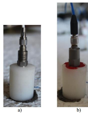
Figure 3.15. Two types of accelerometers; (a) Kistler Group accelerometers, (b) PCB Piezotronics accelerometers
