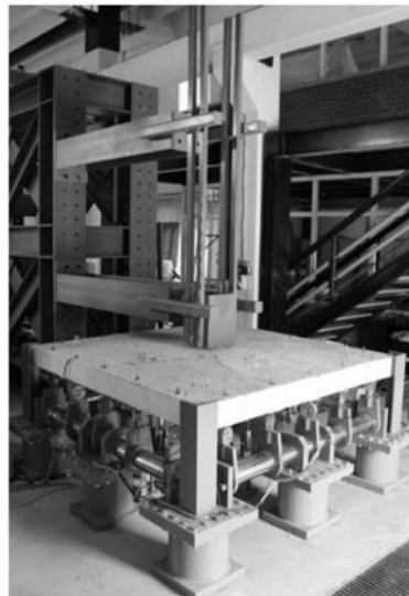
Figure 2.15. Impact test setup (Source: Batarlar, 2013)
