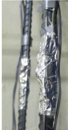
Figure 3.10. Final state of the strain gauge
