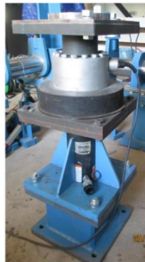
Figure 3.7. Hydraulic piston with 50 ton capacity load cell on top
