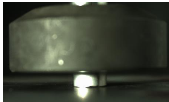
Figure 5.22. Experimentally and numerically deformed pictures of S12 at (a) 0 mm, (b) 4 mm, (c) 6.1 mm, (d) 8.4 mm and (e) 9.1 mm of compressions.
