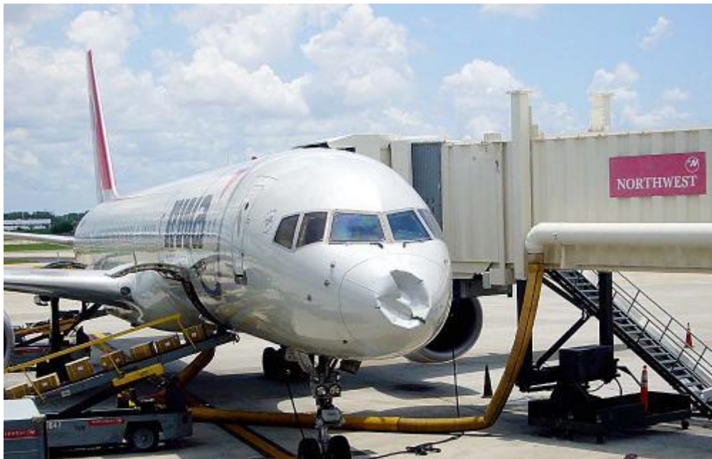
Figure 1.4. The deformed radome of aircraft due to internal structural failure (Source: Welbes 2008).
