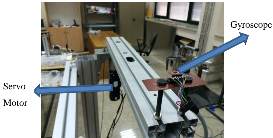
Figure 3.7 Location of the digital gyroscope on the mechanical link
