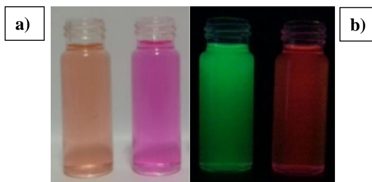
Figure 3.11. a) Day light photograph image of BOD-ZN + Au(III) (left), BOD-ZN (right), (b) fluorescence image of BOD-ZN + Au(III) (left), BOD-ZN (right)
