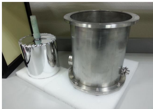
Figure 3.22. Liquid nitrogen reservoir coated with metallized film
