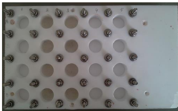
Figure 3.1. Custom made 20 well Teflon mold.
