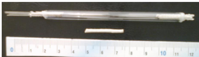
Figure 4.17. General appearance of mold and prepared scaffold.
