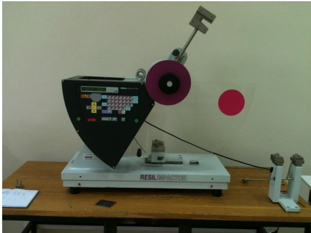
Figure 3.16. Photo of experimental setup for Charpy impact tests
