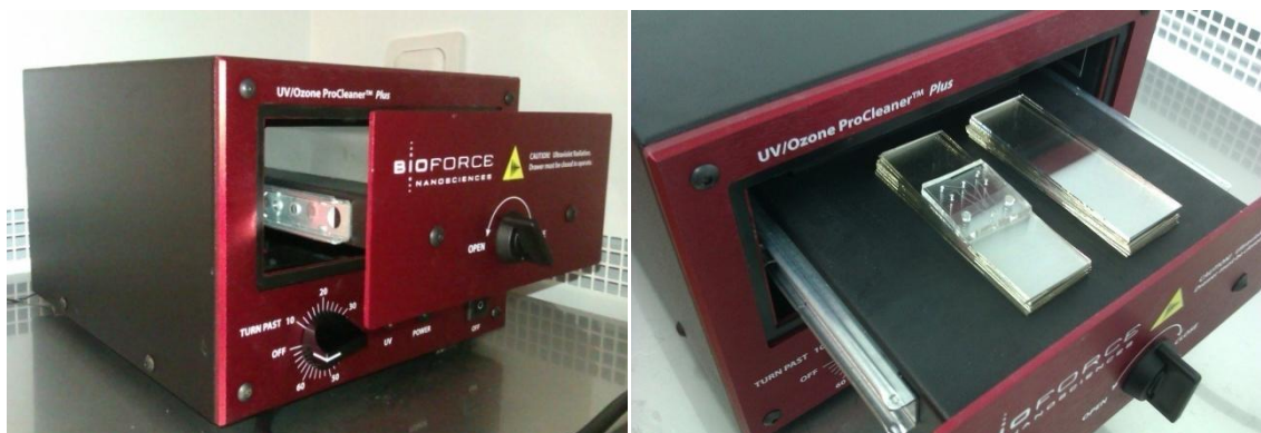
Figure 2.11. The pictures of UV-Ozone used for PDMS bonding.
