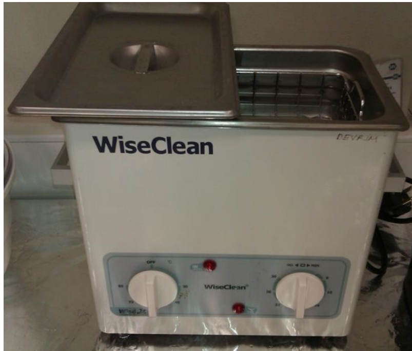
Figure 2.10. The picture of sonicator used for PDMS cleaning.
