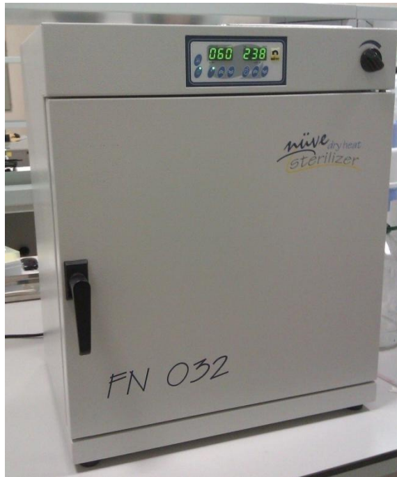
Figure 2.12. The picture of ETUV used for drying sterile cured PDMS and glass coverslips.
