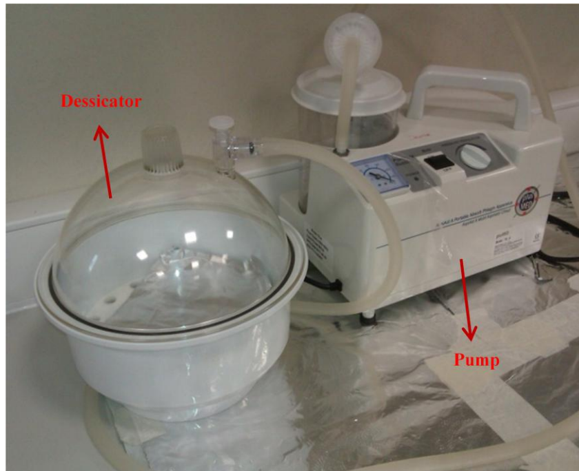
Figure 2.9. The picture of dessicator used for remove any bubble.
