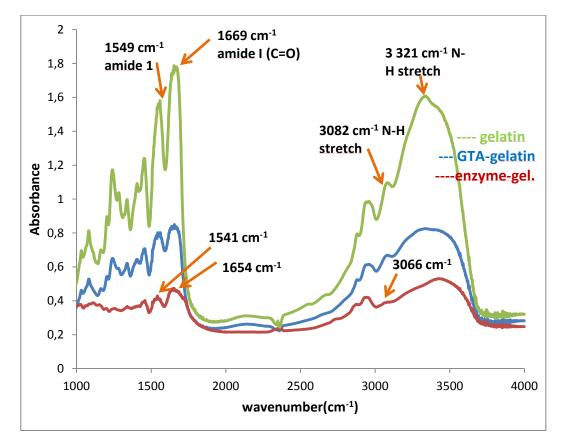
Figure 5.6. The FTIR Spectra of gelatin(----), glutaraldehyde cross linked gelatin (----) and the enzyme entrapped gelatin(----) films.
