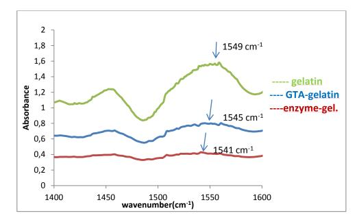
Figure 5.7.The N-H bending vibrations in gelatin(----), glutaraldehyde cross linked gelatin (----) and the enzyme entrapped gelatin(----) films.
