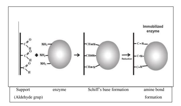
Figure 5.8. Schematic representation of immobilization of enzyme on gelatin support by covalent attachment.
