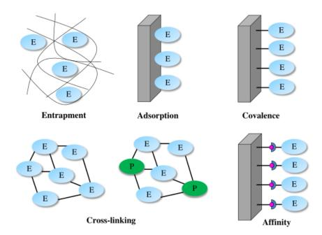
Figure 3.1. Classification of Immobilization Methods (Source: Sassolas, Blum et al. 2012)
