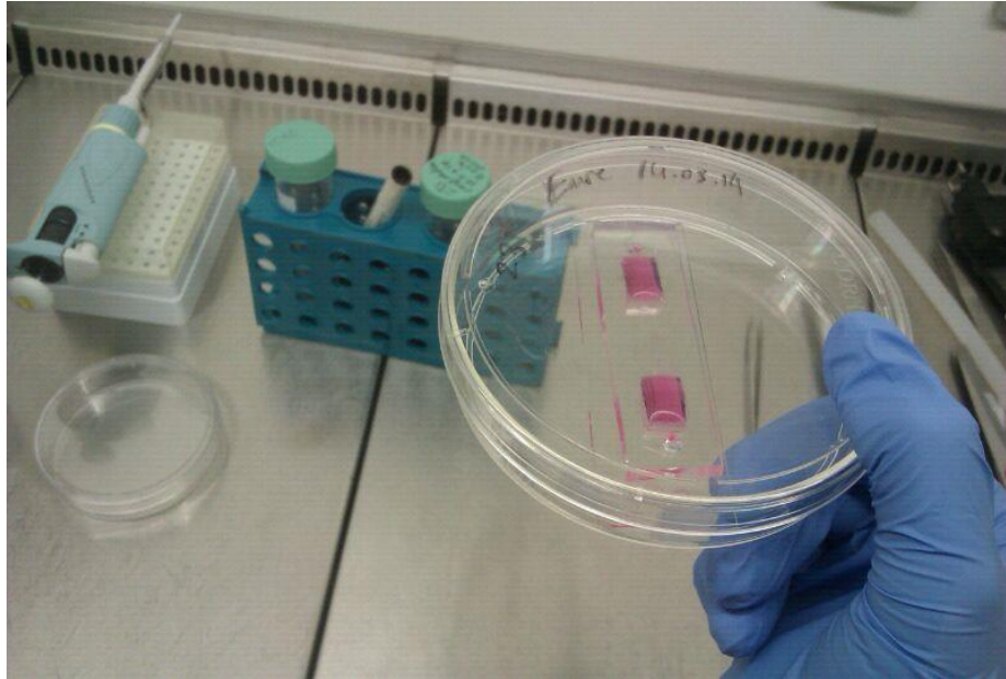
Figure 2.14. Sacrificial material was removed and MBA-MD 231 cell complete medium was filled into the large holes.
