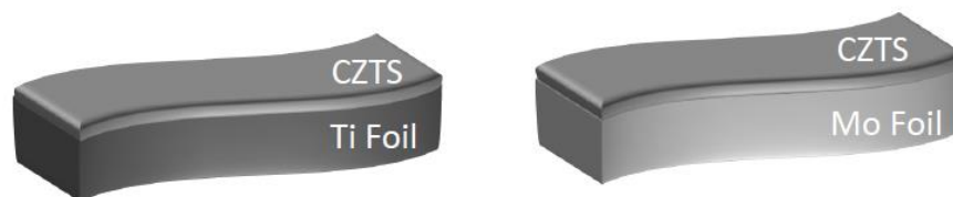
Figure 5.5. Schematic representation of Ti and Mo foil substrate CZTS samples
