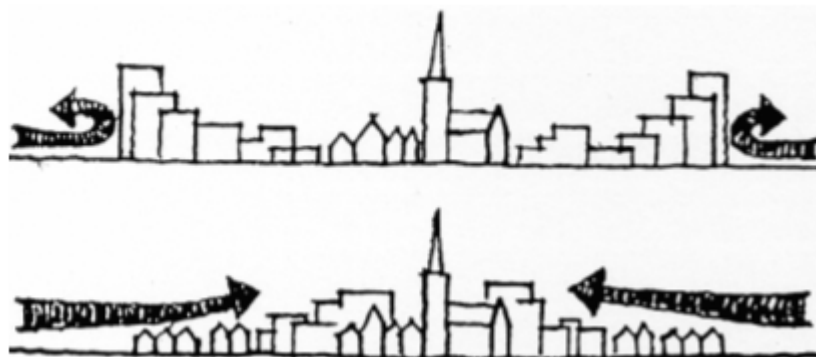
Figure 4.12. The effect of distribution of the buildings with respect to height on wind directions through the city (Source: Ministry of Economy Baden-Württemberg 2008, 5).
