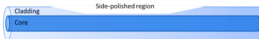
Figure 119. Side-polished optical fibers manufactured by Phoenix Photonics.
