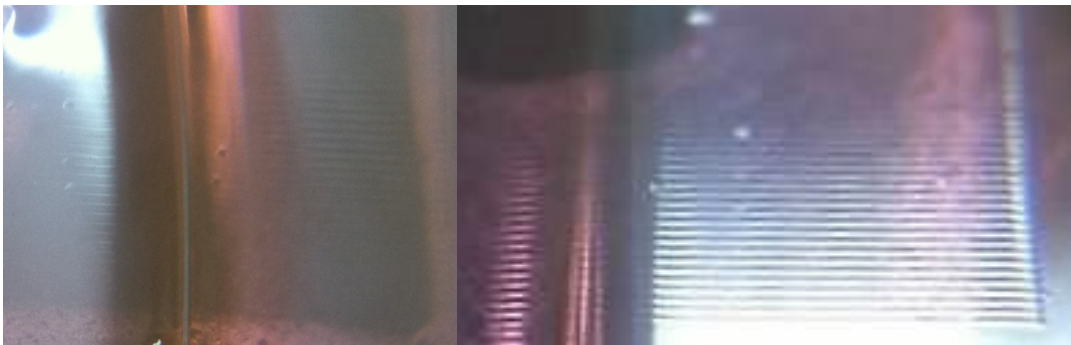
Figure 134. Reflection microscope image of the fiber with the fabricated grating
