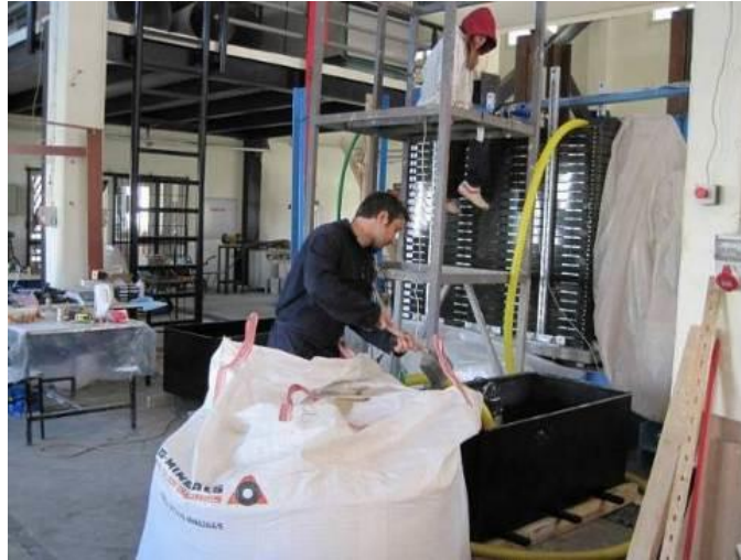
Figure 3. 17. Hydraulic filling process at IZTECH.
