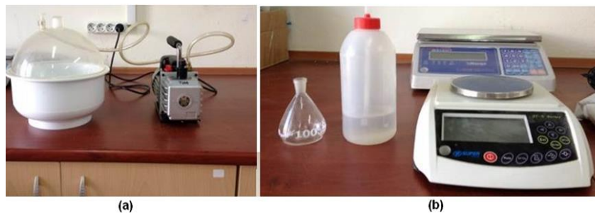
Figure 3. 7. (a) Desiccator and Vacuum Pump, (b) Pycnometer, Distilled Water and Weighting scale (Left to Right).
