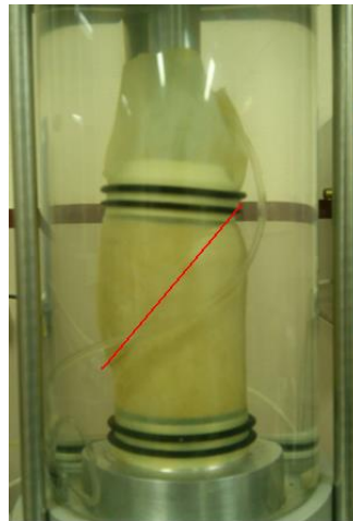
Figure 4. 2. Failure plane of specimen sheared at initial confining stress of 100 kPa.
