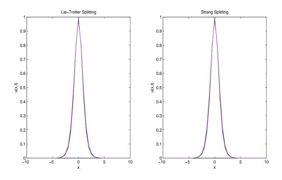
Figure 4.3. Approximate solutions at t=0 to t=0.2 with step size  $\Delta t=0.05$ .
