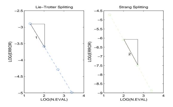
Figure 4.5. Order of the splitting methods for the Fisher's equation.
