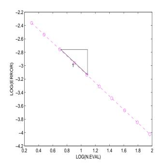
Figure 4.10. Order of the Lie-Trotter splitting for the BBM equation.
