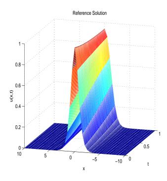
Figure 4.1. Reference solution generated by fourth order Runge-Kutta for  $x \in [-10, 10]$  and  $t \in [0, 1]$ .
