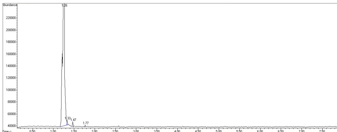
Figure 4.10. GC-MS chromatogram of combustion of sunflower oil by using 20% Ni/56% Mn 2 O 3 /Al 2 O 3 (First Ni precursor added) at 195 °C for 1 h
