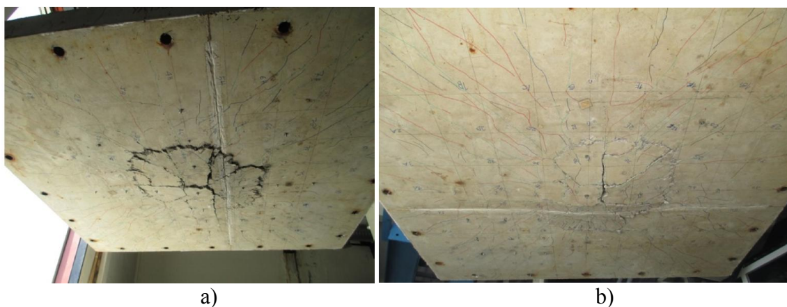
Figure 3.40. a) Formation of punching cone and b) General view of the back face of the specimen YA150fb after testing
