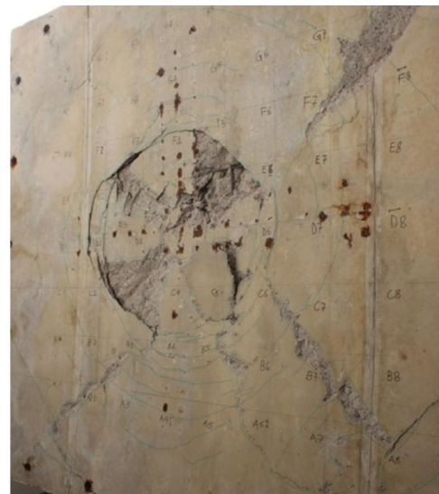
b) Loading face of the specimen YA200a, after testing
