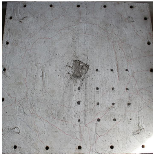
Figure 3.37. Impacted face of the specimen YA150b after tests
