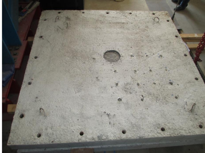
Figure 3.41. Impacted face of the specimen YA150fb after testing
