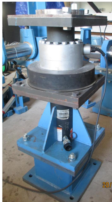
Figure 3.10. Hydraulic piston with 50 ton capacity load cell on top
