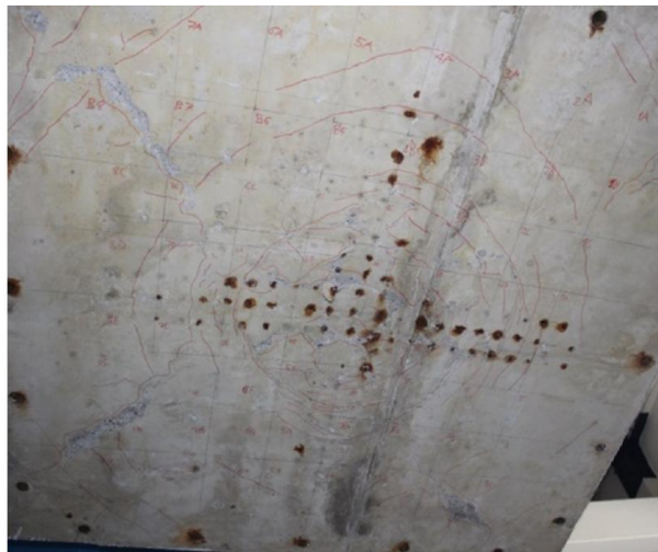
b) Loading face of the specimen YA150a, after testing
