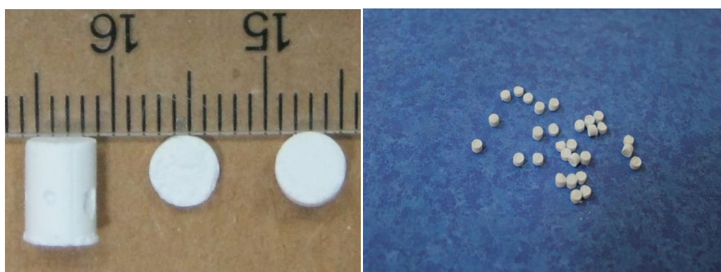
Figure 4.2. The picture of hydroxyapatite cement samples.
