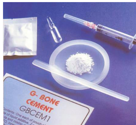
Figure 4.1. The picture of commercial calcium phosphate cement kit (Source: Dorozhkin, 2013).
