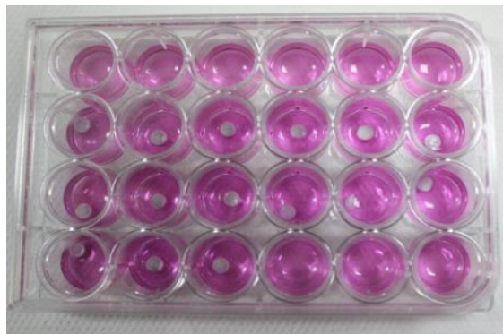
Figure 4.5. HA cement samples in a well plate containing L929 cell culture medium.
