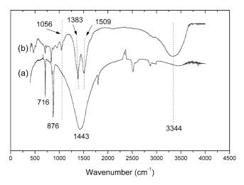
Fig. 7. FTIR spectra of calcite (a) and Zn-loaded calcite after 7 days of contact (b).
