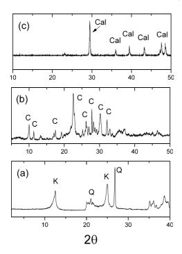
Fig. 1. XRPD patterns of the minerals used in this study, kaolinite (a), clinoptilolite (b), and calcite (c).
