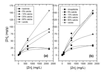
Fig. 3. Variation of the equilibrium concentration on the solid phase with that in the liquid phase for different  $Zn^{2+}$  loadings and mixture compositions: (a) calcite–kaolinite, (b) calcite–clinoptilolite.
