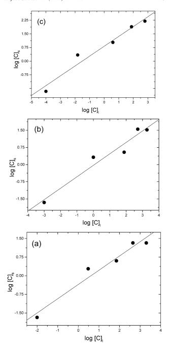
Fig. 2. Freundlich isotherm plots for sorption of  $\mathrm{Zn}^{2+}$  on (a) kaolinite, (b) clinoptilolite, and (c) calcite.
