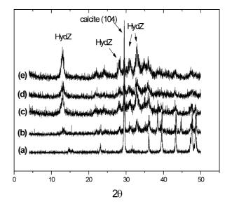
Fig. 5. XRPD diagrams of Zn-loaded calcite, showing the formation of hydrozincite at different contact times, initially (a) and after 7 h (b), 24 h (c), 48 h (d), and 7 days (e).
