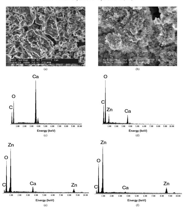
Fig. 6. Typical SEM micrographs of calcite (a), and hydrozincite (b). EDS spectra of Zn-loaded calcite at different contact times: initially (c) and after 1 h (d), 24 h (e), and 3 weeks (f).
