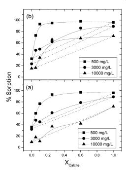
Fig. 4. The change of percentage sorption with the fraction of calcite at initial loadings of 500, 3000, and 10,000 mg/L of Zn(NO<sub>3</sub>)<sub>2</sub>: (a) calcite–kaolinite, (b) calcite–clinoptilolite.
