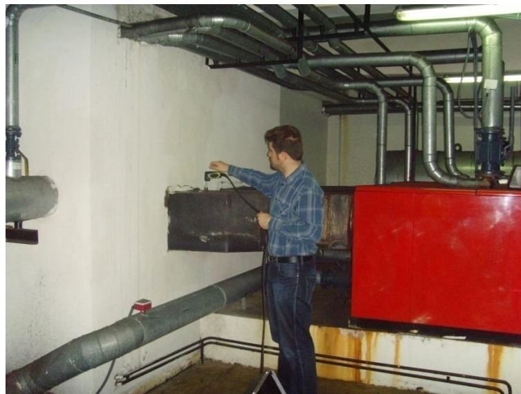
Figure 3.4. Flue gas emission measurement (2008).
