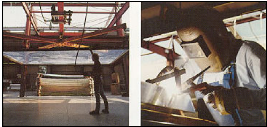
Fig. 3.48. Assembling Pillows And Frames Source: www.texlon.ch
