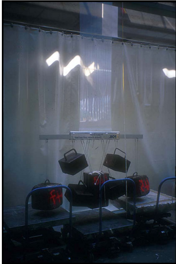
Fig. 3.12. Elongation Tests of ETFE Source: www.vector-foiltec.com
