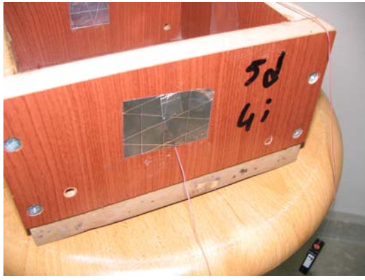
Figure 4.27. MDF Covering, insulator and thermocouples for heat loses measurements
