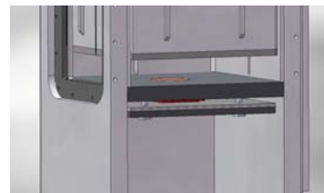
(d) Assembly of heater group into jet set-up
