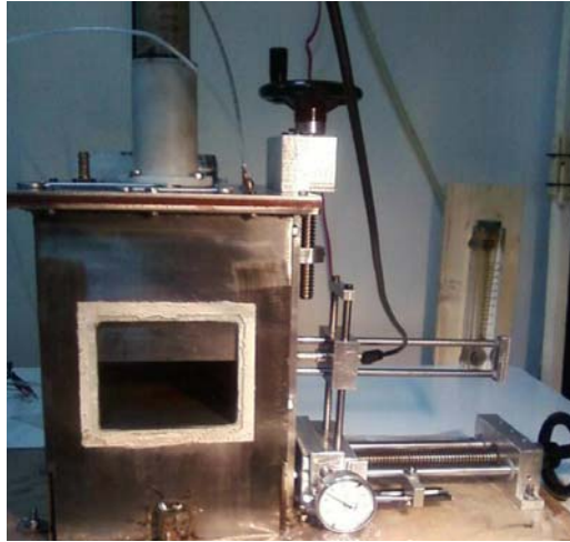
Figure 4.19. Traverse mechanism assembled on the jet set-up and its comparator
