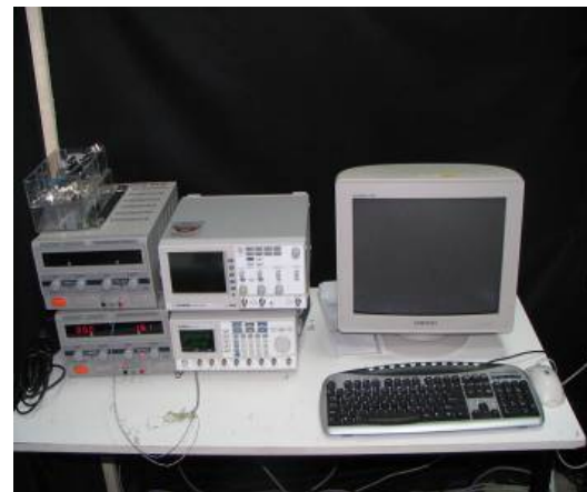
Figure 4.18. Function generator, oscilloscope, power supplies and computer
