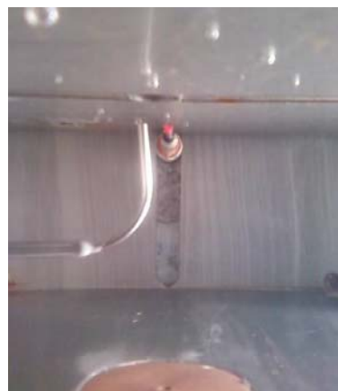
Figure 4.24. Settling of hot wire sensor and pitot tube for calibration
