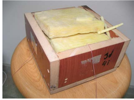
Figure 4.27. MDF Covering, insulator and thermocouples for heat loses measurements
