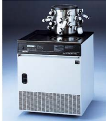
Figure 5.1. The picture of LABCONCO Freeze Dryer used for the preparation of composites in this work
