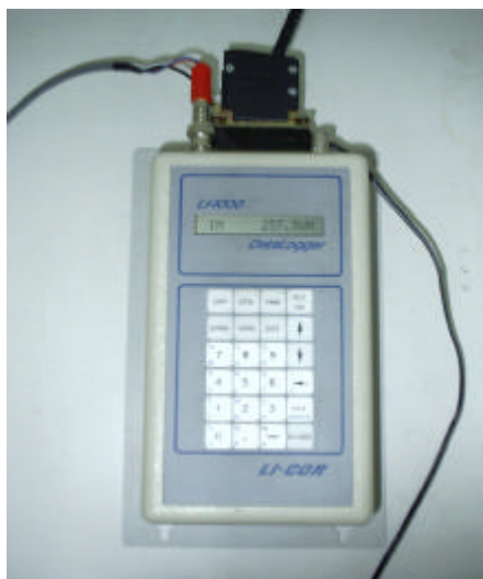
Figure 5.4 LI-1000 Data Logger at the Site[66].
