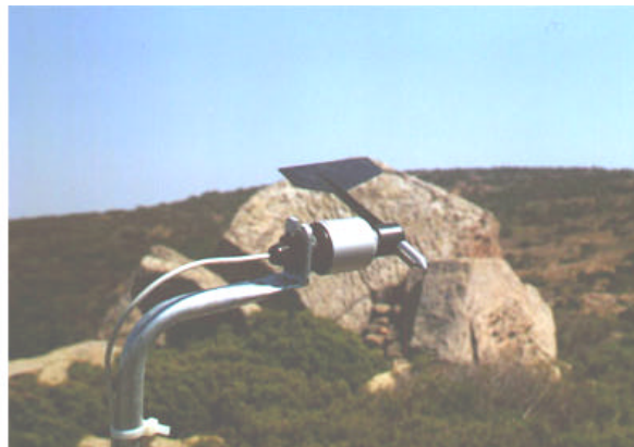
Figure 6.2 Wind Vane at the Site.
