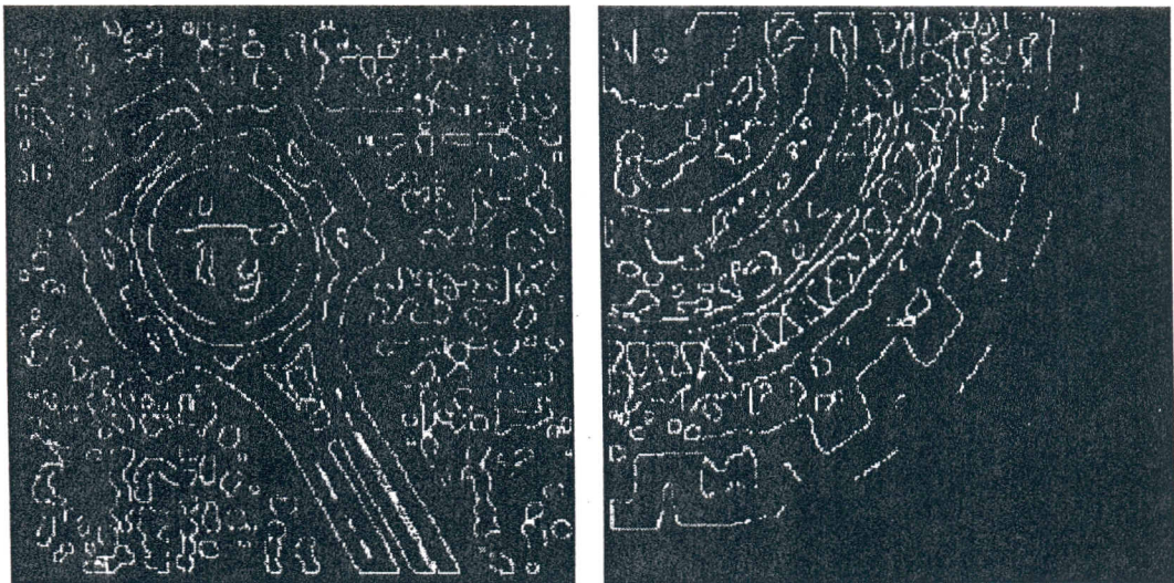
Figure 5-13: Results of Laplacian of Gaussian edge detector.
