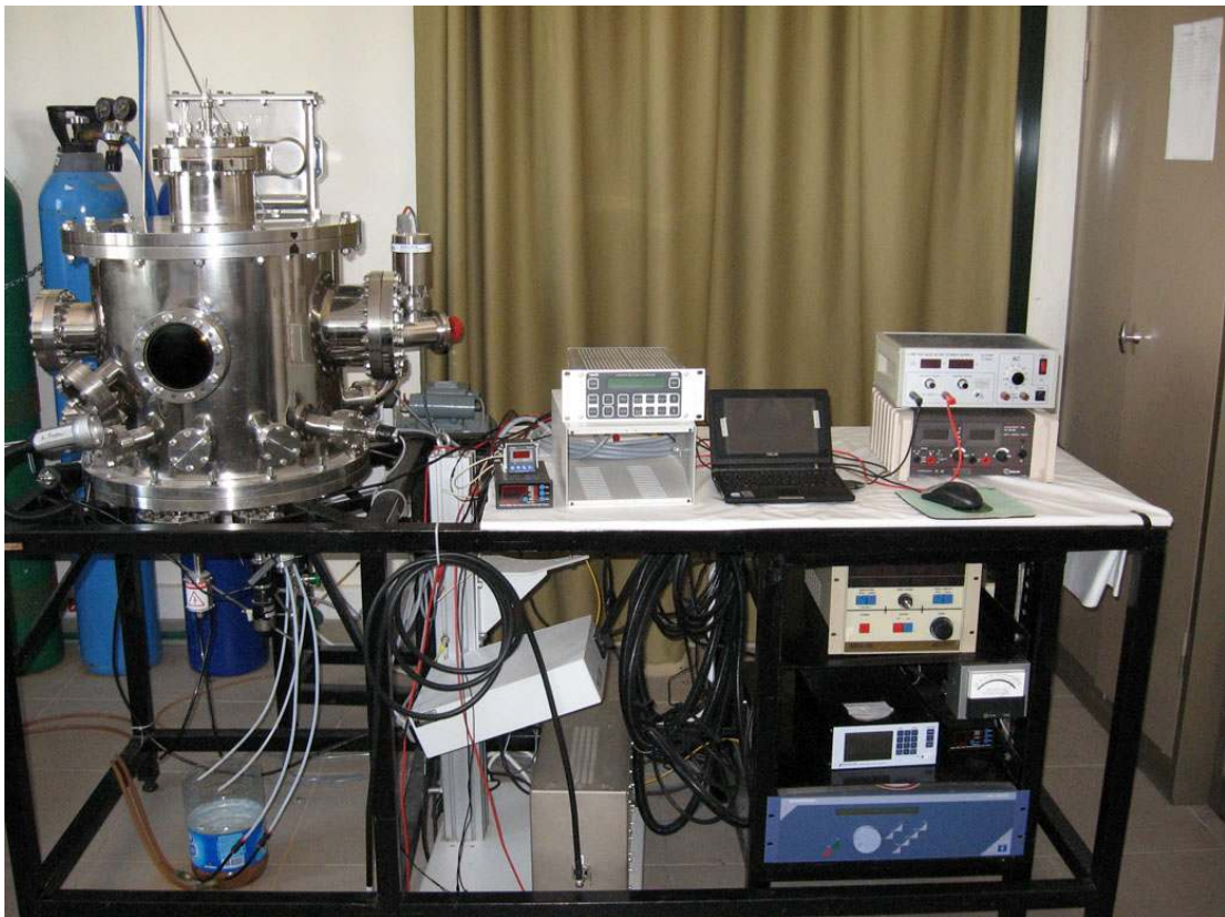
Figure 3.11. Picture of the magnetron sputtering system
