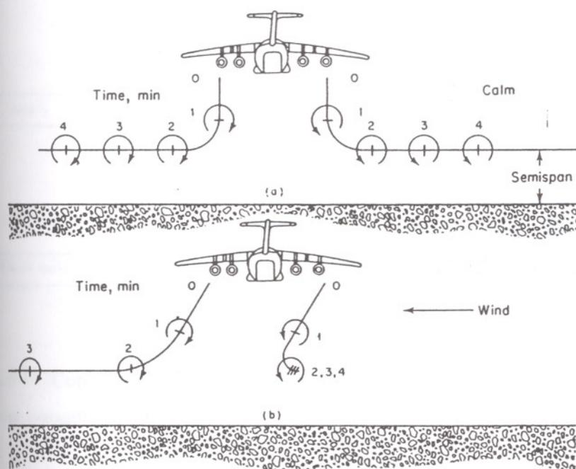
Fig. 4.10 Vortex movement near the ground showing the effect of wind.
