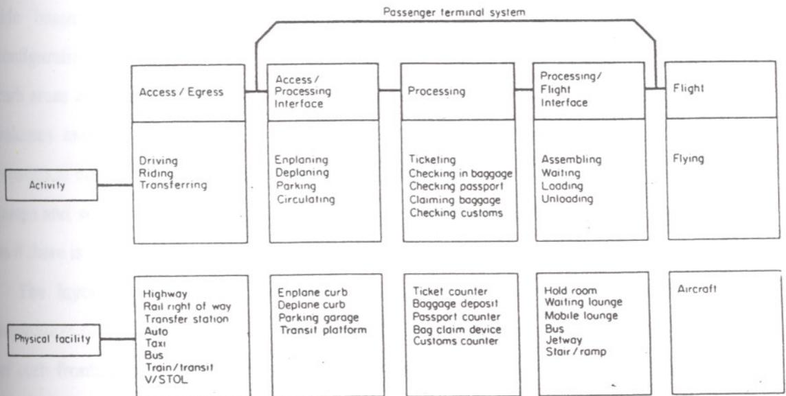
Fig. 4.11 Components of the passenger terminal system
