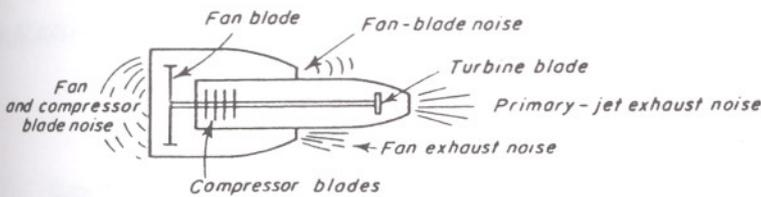
Fig. 4.8 Sources of noise in jet engines
