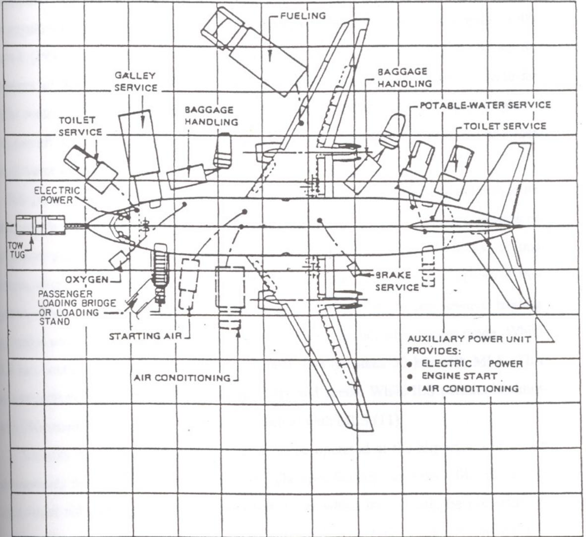
Fig. 4.7 Typical ground equipment service layout
