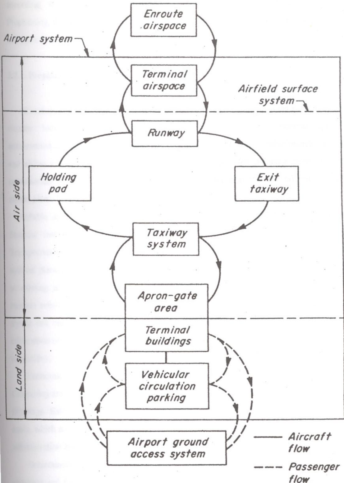
Fig. 3.2 Components of the airport system for a large airport
