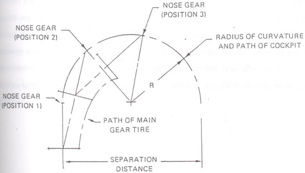
Fig. 4.9 Graphical solution of a 180° turn
