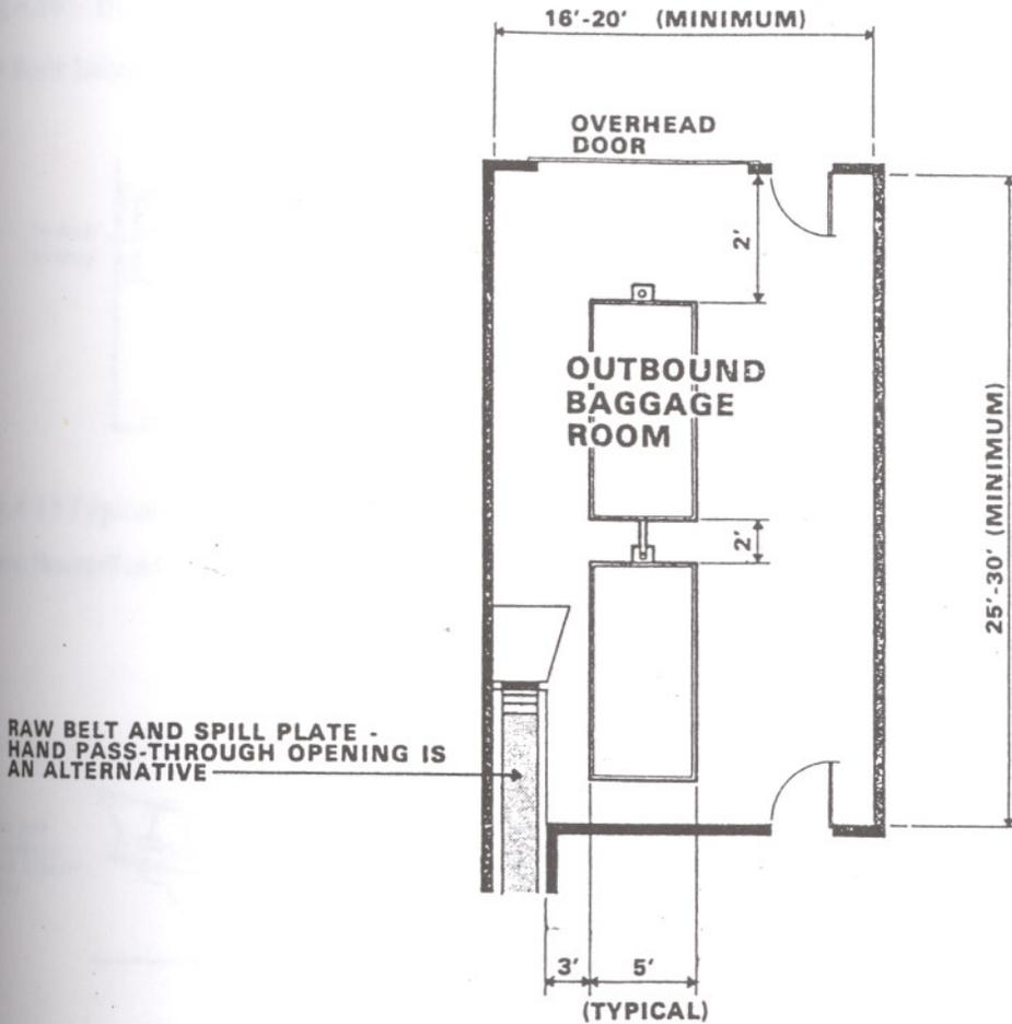
Fig.4.14 Outbound baggage room typical raw belt conveyor installation
