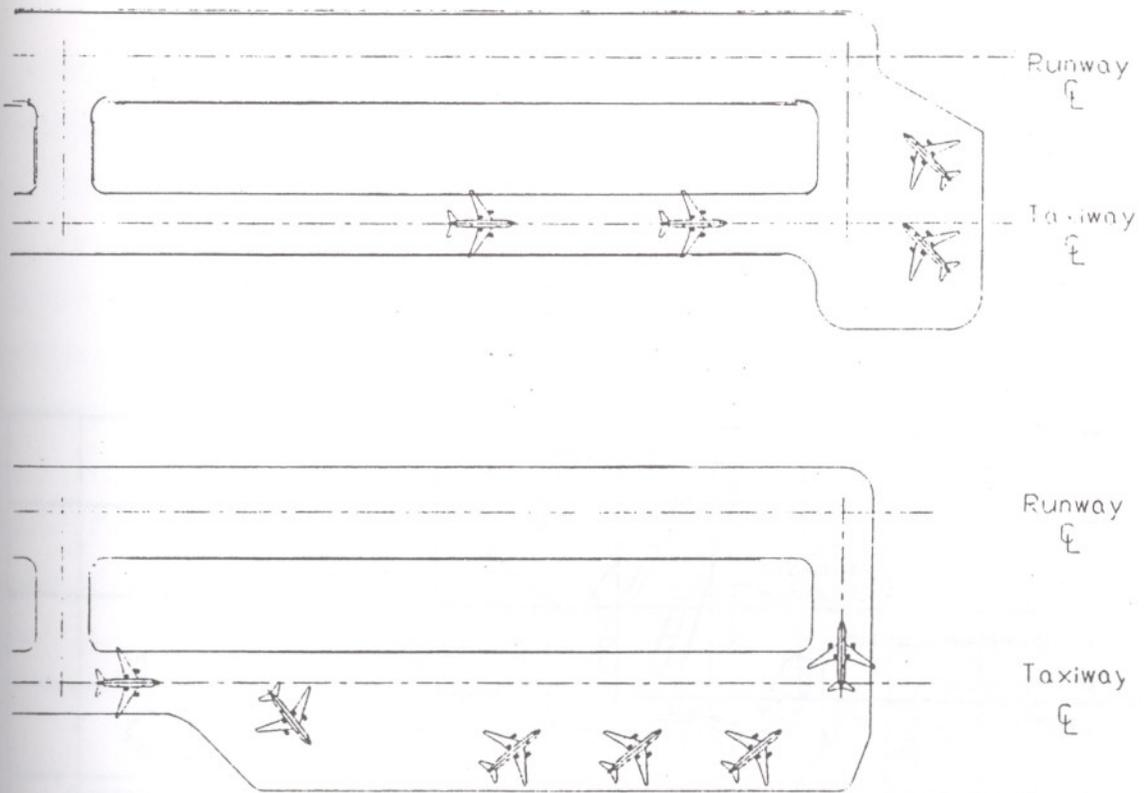
Fig. 4.6. Typical holding pad configurations
