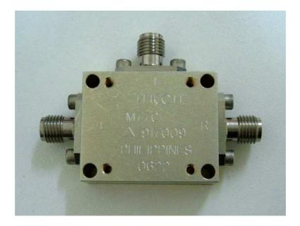
Figure 4.14. View of the commercially available mixer
