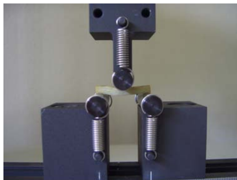
Figure 3.6. SBS test configuration
