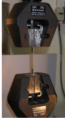
Figure 3.4. Tensile test specimen during the test
