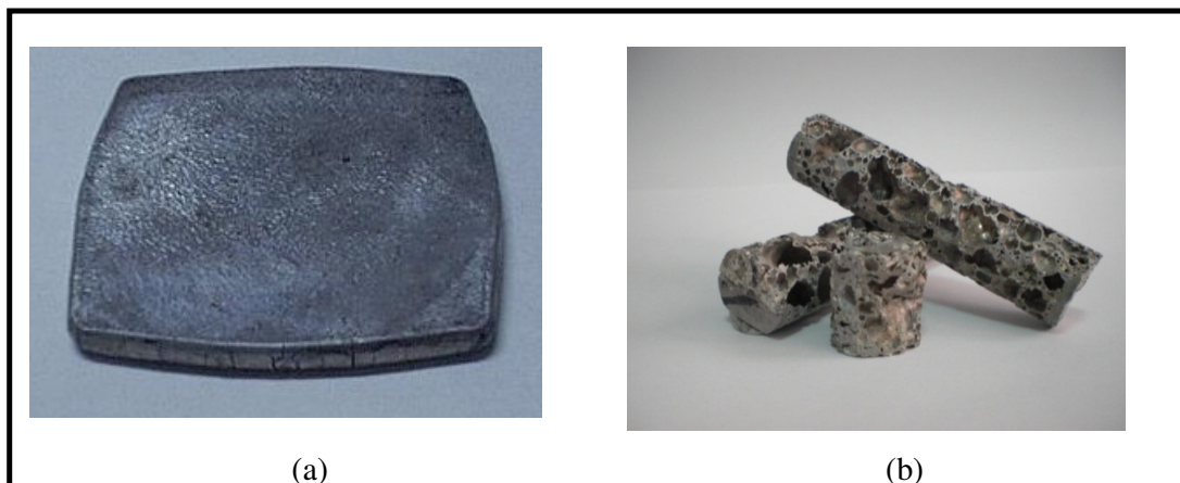
Figure 2.3. Pictures of (a) cold compacted foamable precursor and (b) core-drilled foam plate
