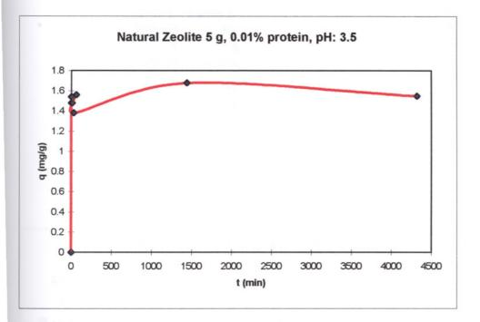
Figure 17. Uptake (q vs.t) Diagram for Natural Zeolite - BSA Pair
