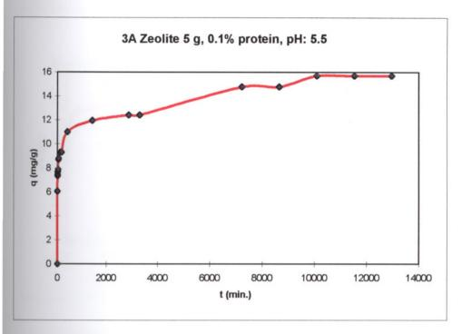
Figure 8. Uptake (q vs.t) Diagram for 3A Zeolite - BSA Pair
