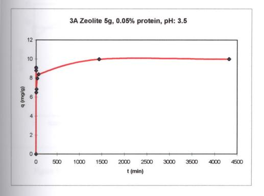
Figure 15. Uptake (q vs.t) Diagram for 3A Zeolite - BSA Pair
