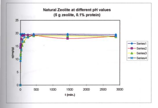
Figure 7. Comparison of q vs. t diagrams of different pH values for natural zeolite
