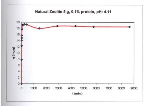
Figure 5. Uptake (q vs.t) Diagram for Natural Zeolite-BSA Pair
