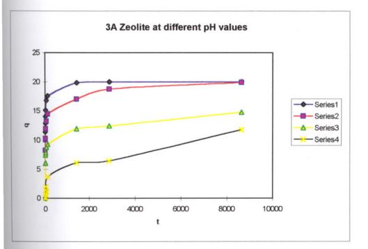
Figure 12. Comparison of q vs. t diagrams of different pH values for 3A Zeolite
