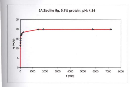
Figure 10. Uptake (q vs.t) Diagram for 3A Zeolite - BSA Pair
