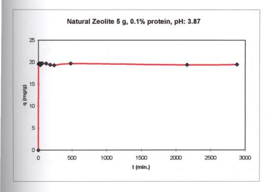
Figure 4. Uptake (q vs.t) Diagram for Natural Zeolite-BSA Pair
