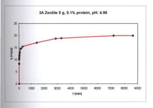
Figure 9. Uptake (q vs.t) Diagram for 3A Zeolite - BSA Pair
