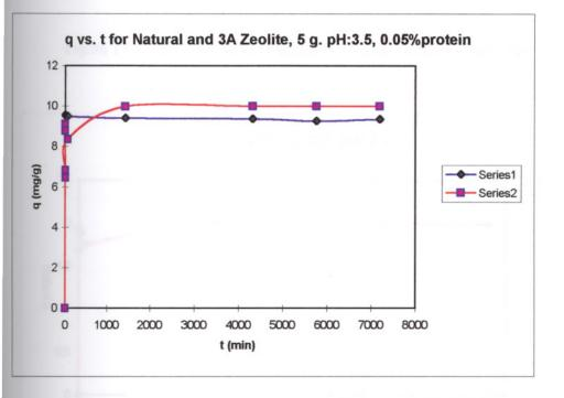
Figure 16. Comparison of q vs. t diagrams for Natural and 3A Zeolite at 0.05% protein concentration
