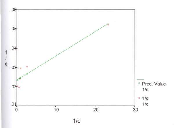
Figure 23. Application of Langmuir Model to describe adsorption isotherms for clinoptilolite with the use of SPSS Statistical Program.
