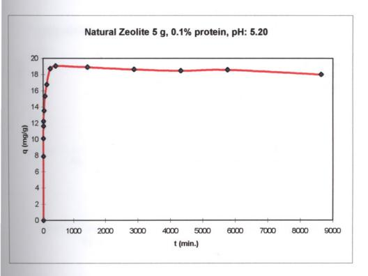
Figure 6. Uptake (q vs.t) Diagram for Natural Zeolite-BSA Pair
