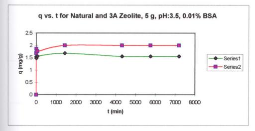
Figure 19. Comparison of q vs. t diagrams for Natural and 3A Zeolite at 0.01% protein concentration
