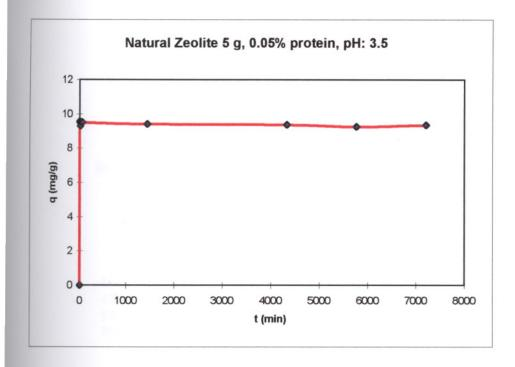
Figure 14. Uptake (q vs.t) Diagram for Natural Zeolite - BSA Pair
