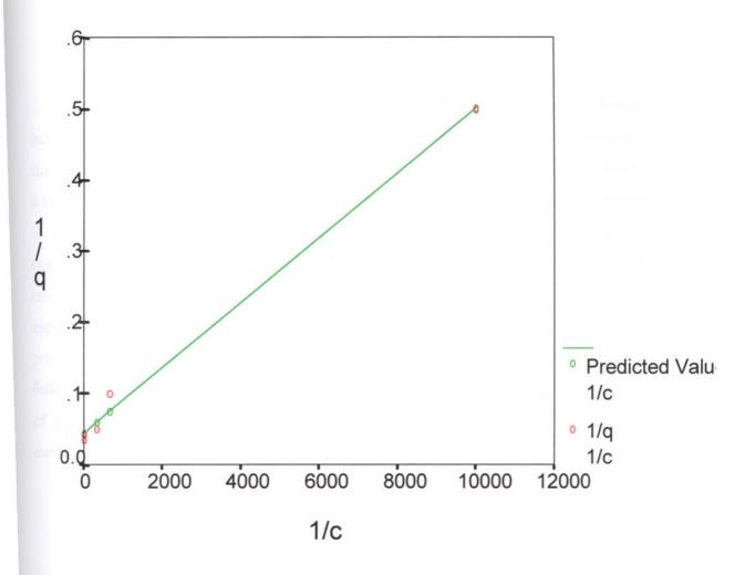
Figure 24. Application of Langmuir Model to describe adsorption isotherms for 3A Zeolite with the use of SPSS Statistical Program.
