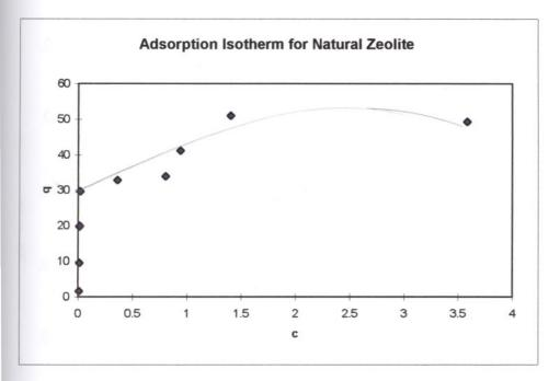
Figure 21. Adsorption isotherm for natural zeolite
