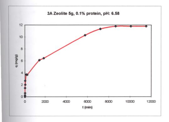
Figure 11. Uptake (q vs.t) Diagram for 3A Zeolite - BSA Pair
