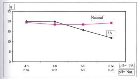
Figure 20. Effect of pH on BSA Adsorption
