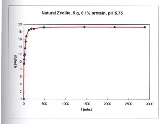
Figure 3. Uptake (q vs.t) Diagram for Natural Zeolite-BSA Pair
