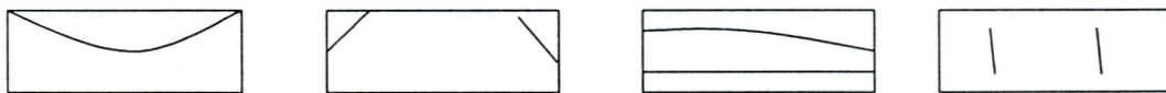
Figure 5.3 Illustrations of typical end capping, ring capping, lamination, and vertical crack defects in cross-sections of cylindrical powder compacts pressed uni-axially from the top to down [45].
